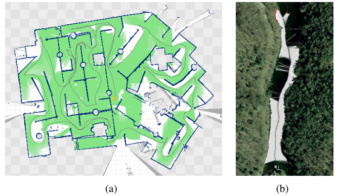
Fig. 5. Vehicle experiments: (a): Map learned at the RoboCup 2010 competition. (b) Learned grid map of 0.25m resolution overlaid over satellite imagery (© Google, Commonwealth of Virginia)
